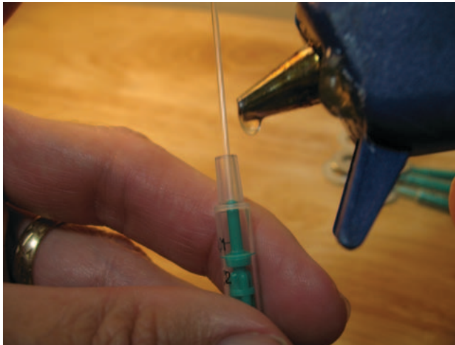
Figure 3. Hot Glue Added to Capillary Tube Base
